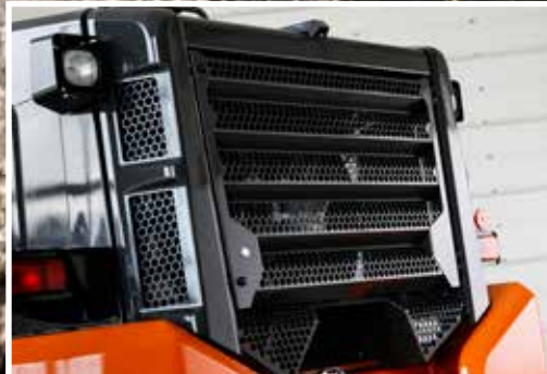
New rear grill protects radiator compartment.
